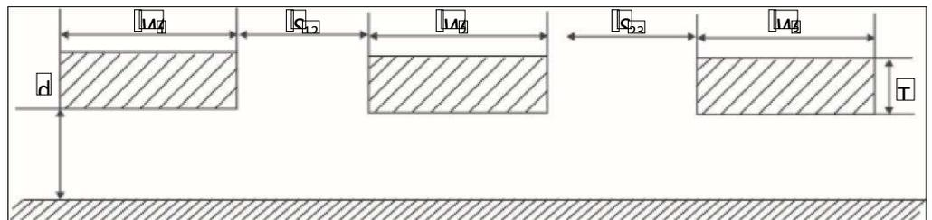
**Fig 1:** Cross Section of Three Conductor Strip Line
